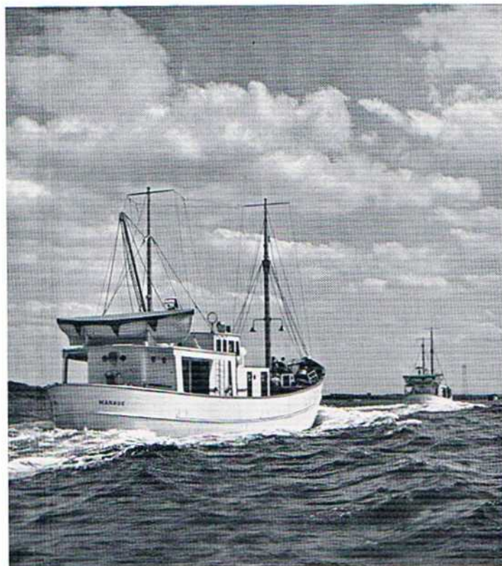
Two specially built 60-GRT refrigerator boats, the „Coronel Medeiros“ and the „Velho Lino“, each designed to carry 12,000 litres of milk on the Amazon, Brazil, have been equipped with 4-cylinder B & W ALPHA diesel engines of the type 400 VO with controllible pitch propellers. The output of each engine is 280/310 BHP at 375 rpm.
