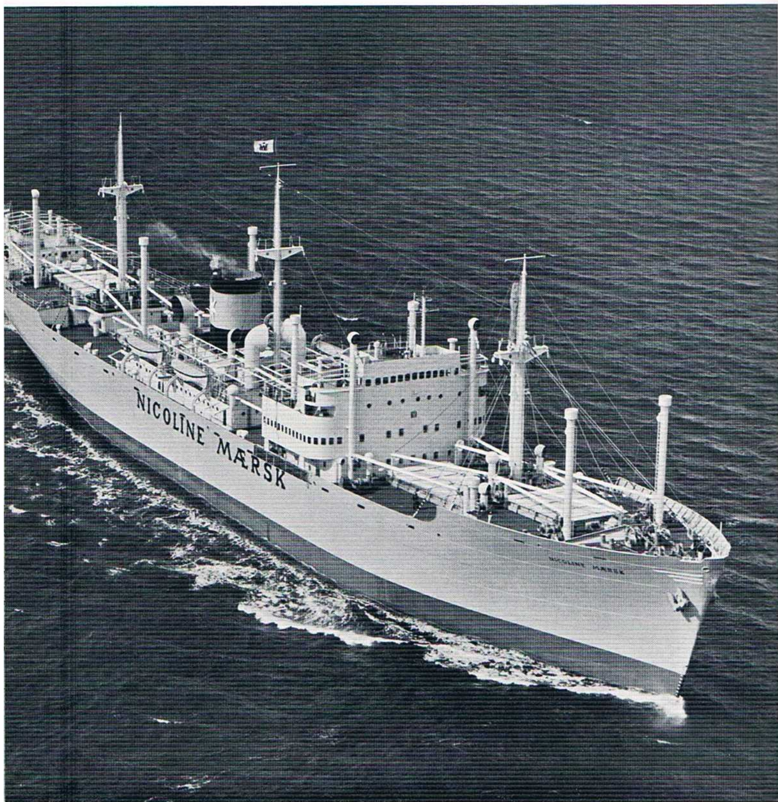
M/S "Nicoline Maersk", cargo motor ship, 9,650 tons dw, built for A. P. Moller, Copenhagen. Length 135.6 m (445'0"), breadth 19.4 m (63'6"), depth 12.7 m (41'6"). The main engine is a 2-stroke, single-acting, 10-cylinder crosshead engine. Cylinder diameter 740 mm, length of stroke 1,600 mm. Normal output 11,500 IHP at 115 rpm. Speed on loaded trials 17.25 knots.
