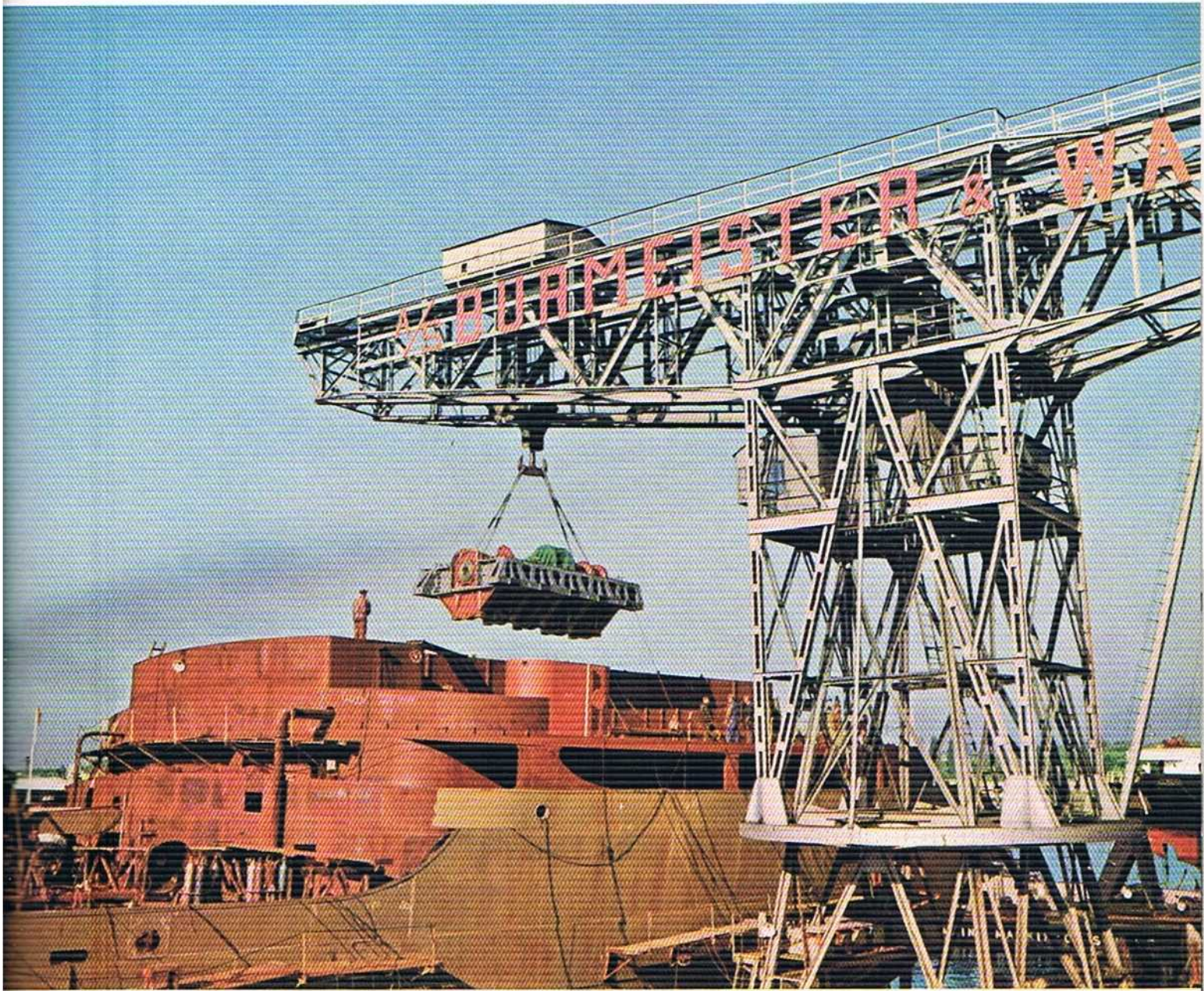
The bedplate of a B & W diesel engine being swung on board a newbuilding at B & W's shipyard on Refshale Island.
