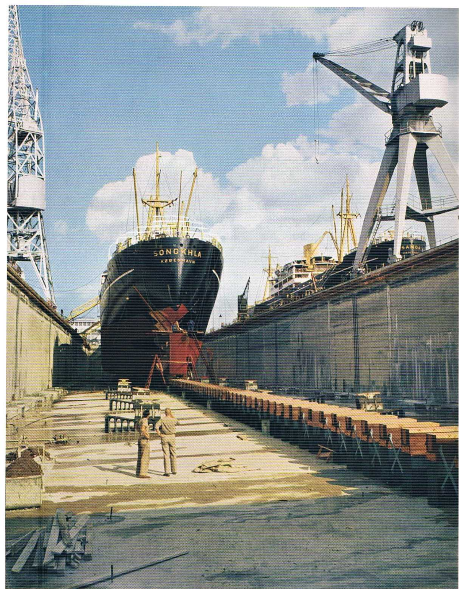
M/S "Songkhla", cargo motor ship, 10,340 tons dw, built for The East Asiatic Company, Copenhagen. Length 139.0 m (456'0"), breadth 19.1 m (62'6"), depth 11.6 m (38'3"). The main engine is a 2-stroke, single-acting, 7-cylinder crosshead engine with turbocharge. Cylinder diameter 740 mm, length of stroke 1,600 mm. Normal output 9,870 IHP at 115 rpm. Speed on loaded trials 16.8 knots.
