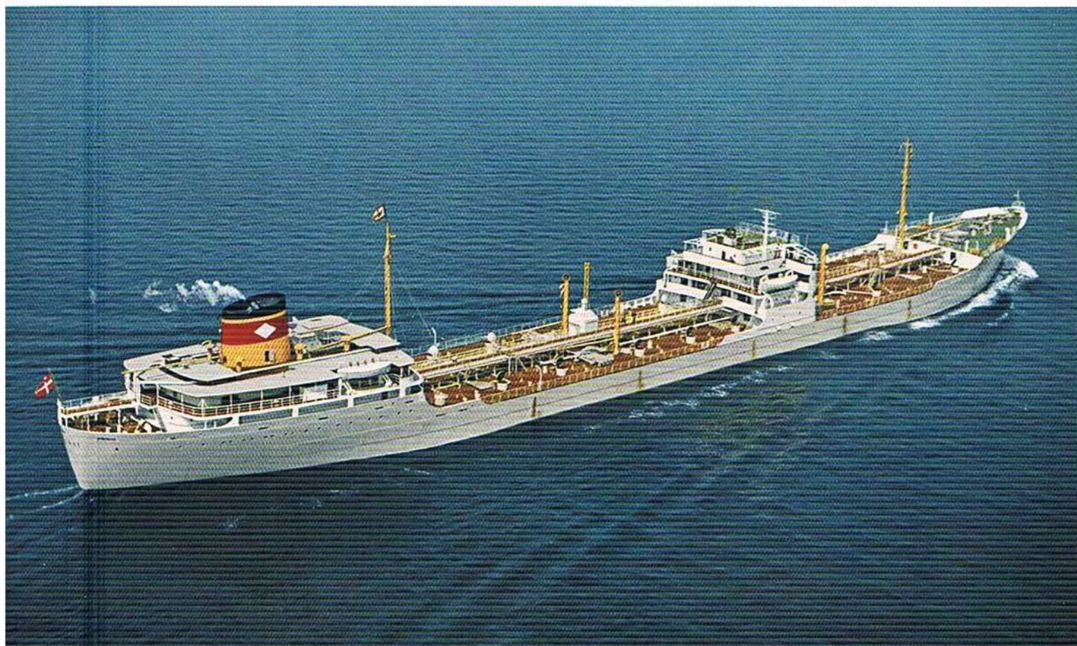
M/T "Dagali", motor tanker, 19,150 tons dw, built for A/S Ocean, Oslo, Norway. Length 166.1 m (545'0"), breadth 21.5 m (70'6"), depth 11.9 m (39'0").
