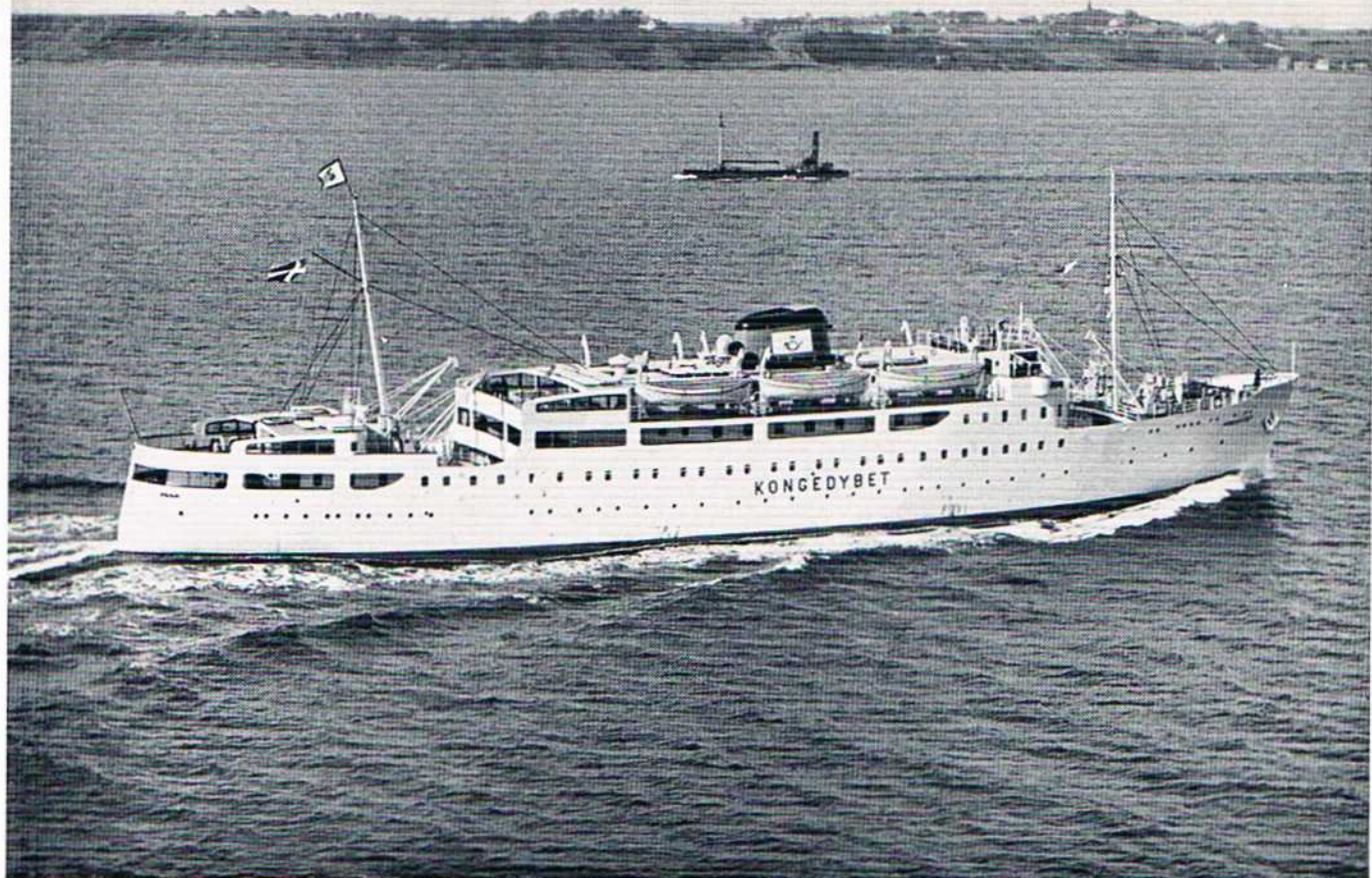
M/S "Kongedybet", passenger and cargo motor ship, 2,310 GRT, built for A/S Dampskibsselskabet paa Bornholm af 1866, Rønne, Denmark. Length 81.9 m (269'0"), breadth 13.3 m (43'6"), depth 5.2 m (16'11").
