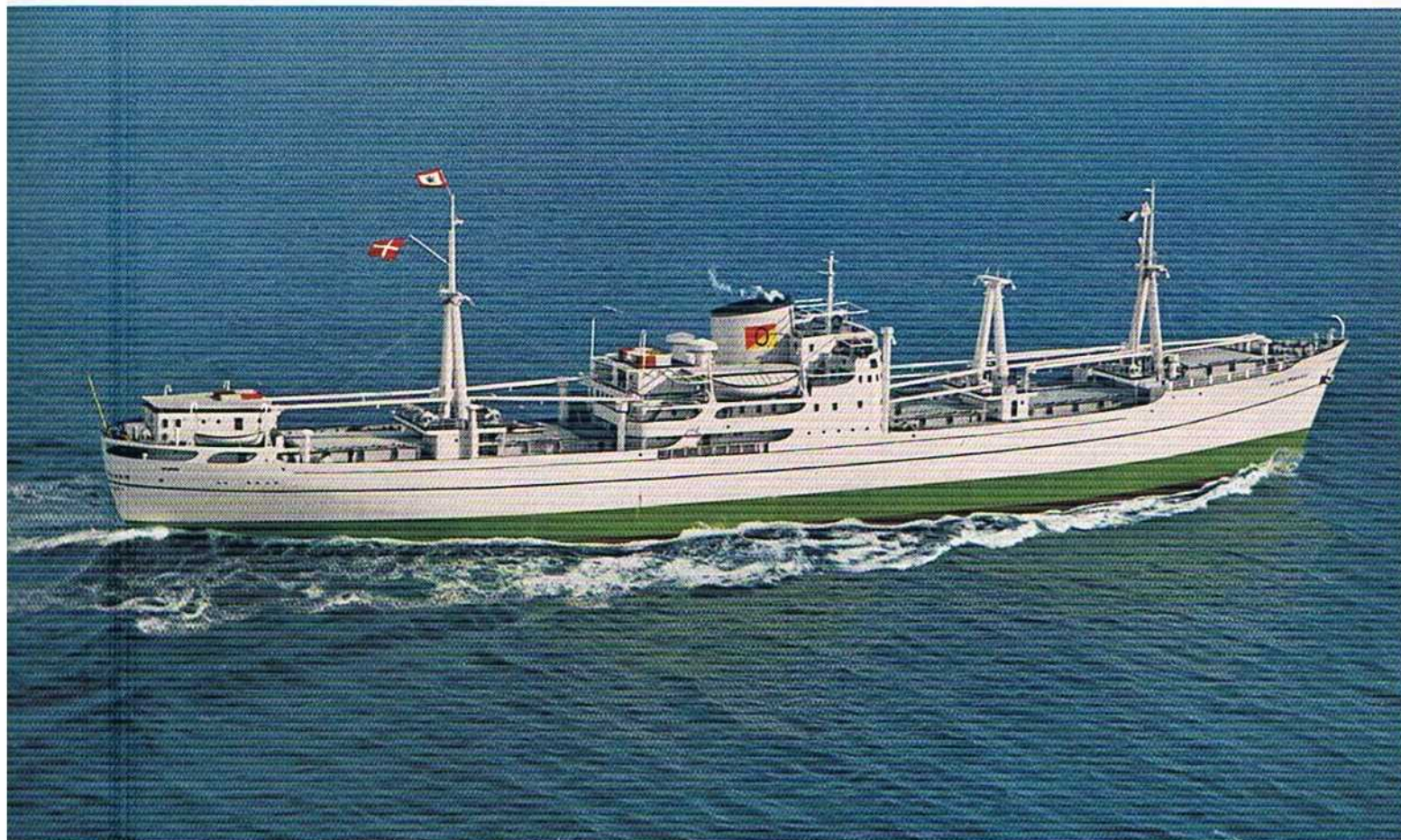
M/S "Thor Odland", cargo motor ship, 7,050 tons dw, built for A/S Produce, Haugesund, Norway. Length 121.9 m (400'0"), breadth 17.2 m (56'6"), depth 10.8 m (35'6").
