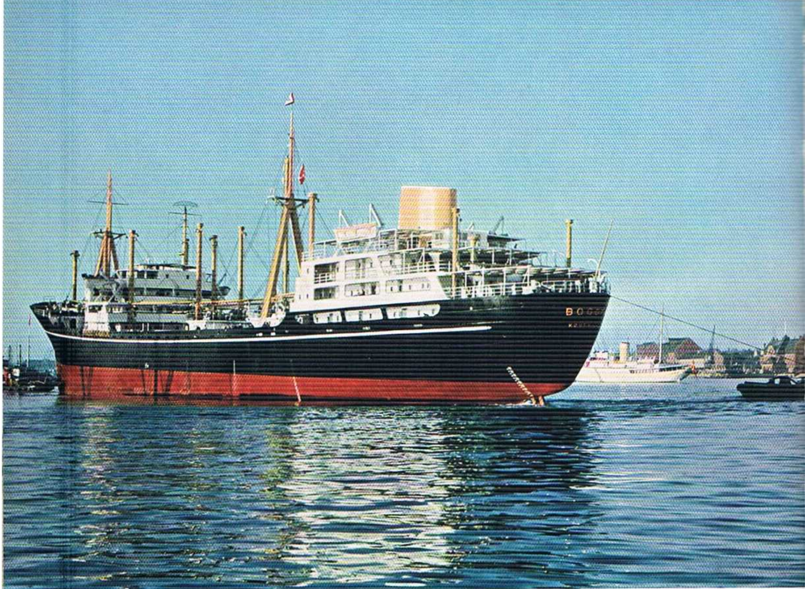
M/S "Bogotá", cargo motor ship, 10,200 tons dw, built for the East Asiatic Company, Copenhagen. The main engine is a 2-stroke, single-acting, 8-cylinder crosshead engine of welded construction, with turbocharge. Cylinder diameter 740 mm, length of stroke 1,600 mm. Normal output 11,100 IHP at 115 rpm. Speed on loaded trials 17.5 knots. M/S "Bogotá" is the first large Danish-built cargo motor ship with engine room aft.
