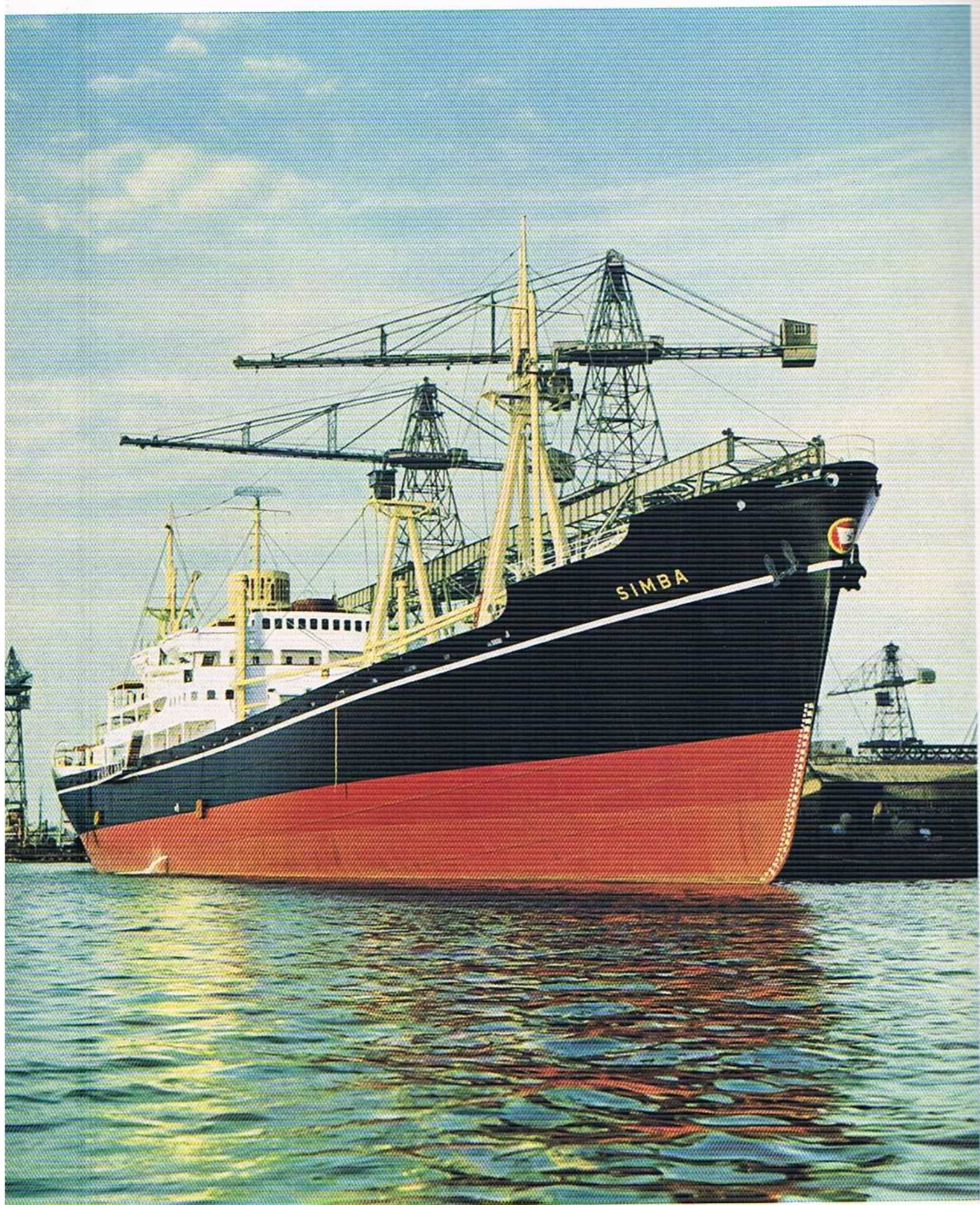
M/S "Simba", cargo motor ship, 10,300 tons dw, built for The East Asiatic Company, Copenhagen. Length 139.0 m (456'0"), breadth 19.1 m (62'6"), depth 11.6 m (38'3"). The main engine is a 2-stroke, single-acting, 7-cylinder crosshead engine with turbocharge. Cylinder diameter 740 mm, length of stroke 1,600 mm. Normal output 9,870 IHP at 115 rpm. Speed on loaded trials 16.8 knots.
