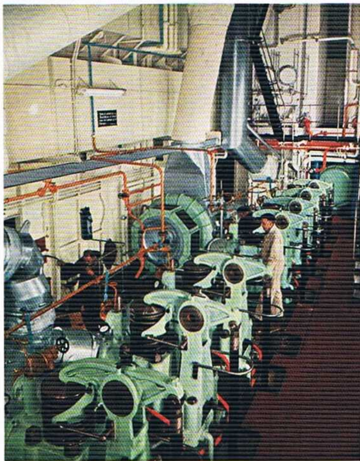
Top of a large B&W main engine with turbocharge. One of the B&W turbochargers is to be seen in the middle of the picture.
